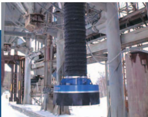
Access to filter inserts for maintenance is straightforward and the filter can be adjusted to meet requirements.
