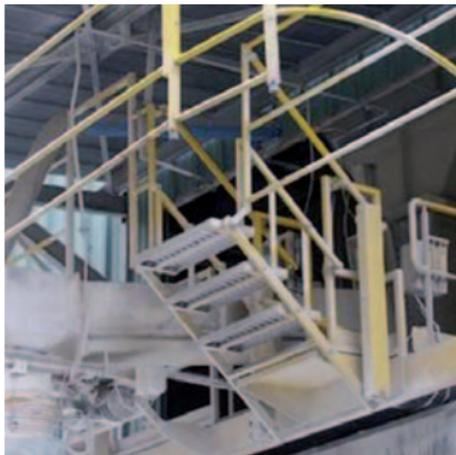
**LISTENOW** supplies **LIS-klap** safety folding steps with 3, 4, and 5 steps to give operators easy access to vehicles, such as tankers, silo trucks and tank wagons.
